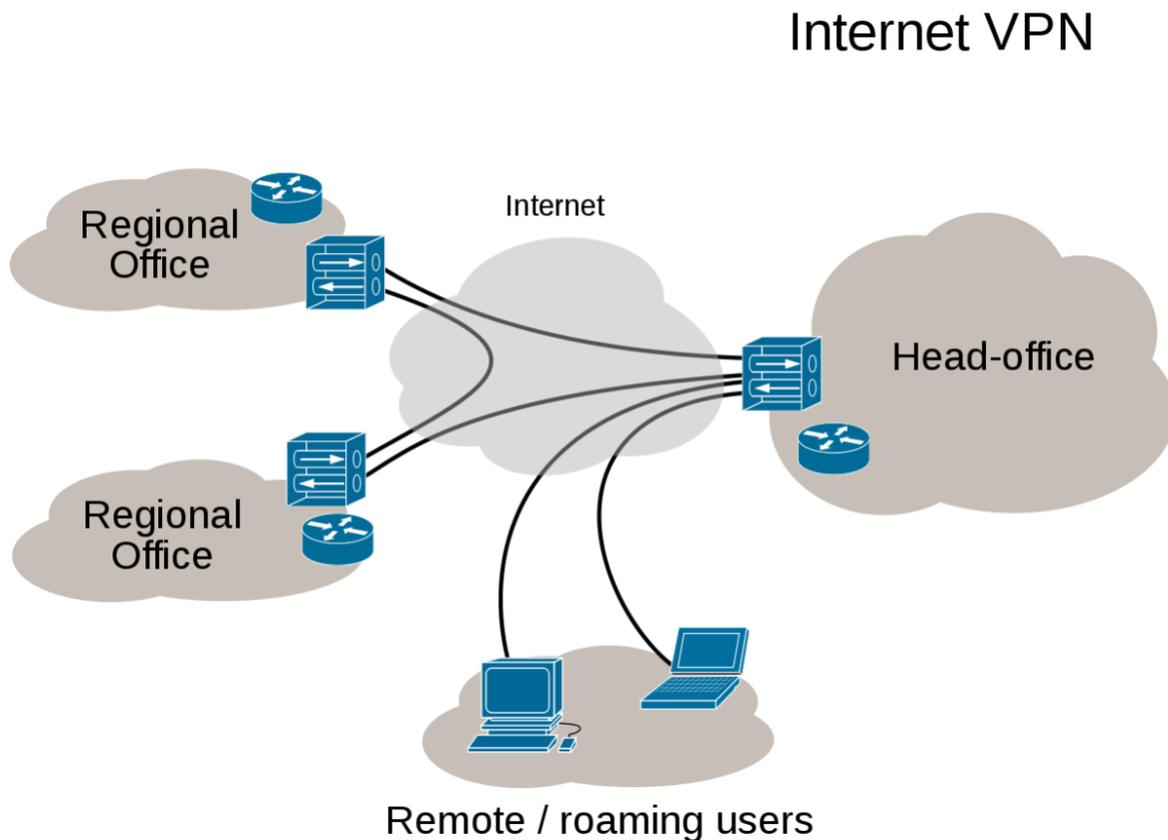
A VPN is created by establishing a virtual point-to-point connection through the use of dedicated connections, virtual tunneling protocols, or traffic encryption. A VPN available from the public Internet can provide some of the benefits of a wide area network (WAN). From a user perspective, the resources available within the private network can be accessed remotely.
